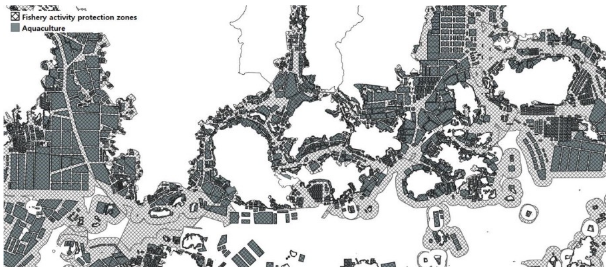
Figure D19. Overlay analysis of aquaculture spatial data (with 1km buffer) and fishery activity protection zones in the case study area
