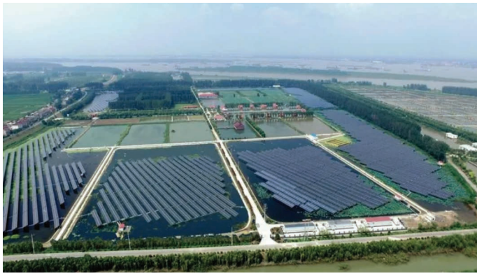
FIGURE 3. The integration of renewable energy systems and aquaculture is developing rapidly. Pictured is an aerial view of the integrated 200 MW solar energy-fish farm in Zhejiang Province, China. Another 120 MW project is also operational in Jiangxi Province, and more are planned.
